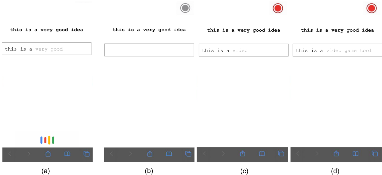
Figure 10: Real-time visual feedback provided by (a) the default Google Speech recognizer and (b–c) MELDER. In (b), the gray circle in the top-right corner indicates that MELDER is unable to track the lips, passively prompting the user to reposition the device for a better camera view. In (c), MELDER is providing word-level feedback and in (d) it is providing phrase-level feedback. The suggestions are in a greyed-out font. In both (c) and (d), the red blinking circle indicates that MELDER is able to track the lips.
